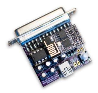
Paul Rickards ( @paulrickards ) has designed a new Hayes Compatible modem that hooks up to retro computers like the TI-99/4A, Atari, Amiga and various other computers via the standard RS-232C connector (DCE) and utilizing the ESP8266 WiFi module.
